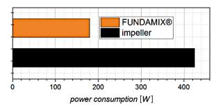
Figure 2: The same FUNDAMIX® and impellers were used as in Fig. 1, running at an amplitude of 2.3 mm and a rotational speed of 500 rpm, respectively [1].
