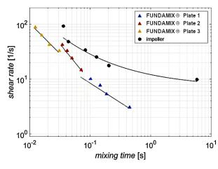
Figure 3: A FM-1 with type A plates of diameters 22, 45, and 65 mm was tested at 100 Hz and amplitudes of 1, 1.5, 2, and 2.5 mm. The data was compared with a 4-blade glass impeller (IKA) with 29 mm diameter, running at 50 – 2'000 rpm [2].
